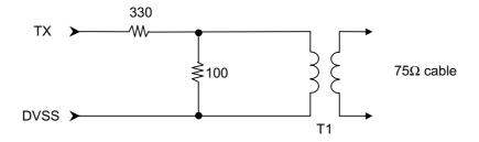
Figure 7. TX External Resistor Network
