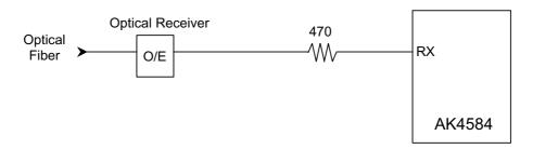
Figure 6. Consumer Input Circuit (Optical Input)
