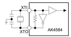
Figure 2. X'tal mode - Note: External capacitance depends on the crystal oscillator (Typ. 10-40pF)
