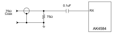
Figure 5. Consumer Input Circuit (Coaxial Input)
