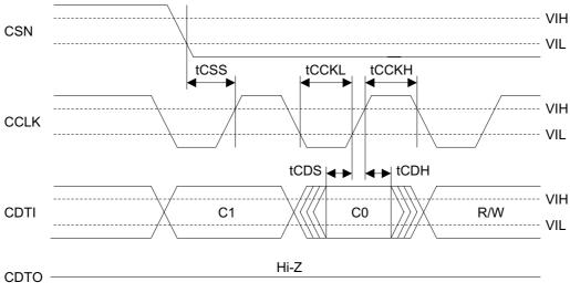
WRITE/READ Command Input Timing
