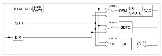
Figure 1. Connection between Input Sources & Output Sources
