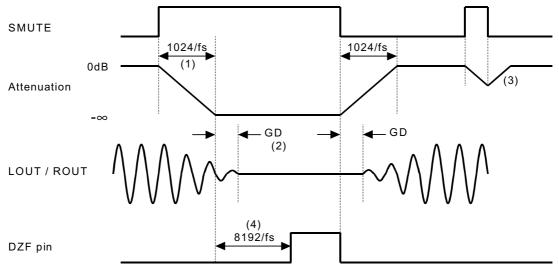
Figure 16. Soft mute function and Zero detection function
